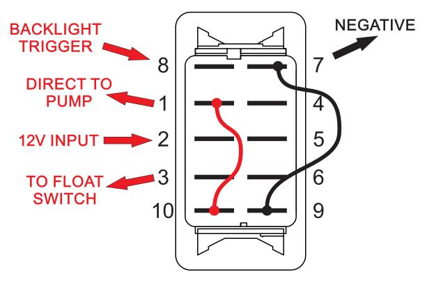
One jumper required between terminals 1 and 10 (positive) One jumper required between terminals 7 and 9 (negative)
